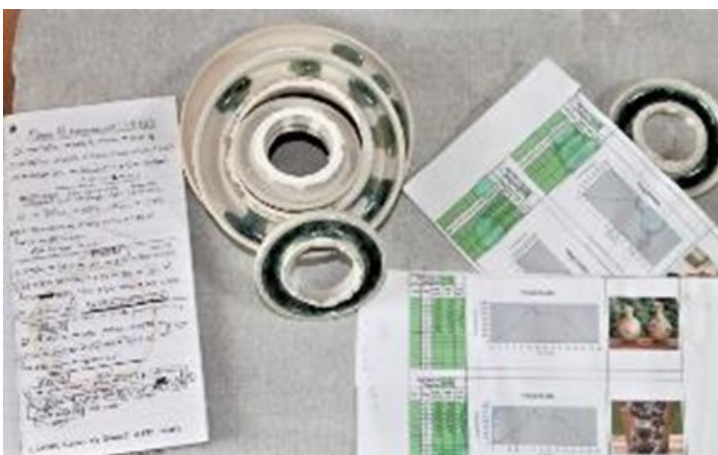
Pots fired upside down to allow glaze runoff to be caught in the rim.
