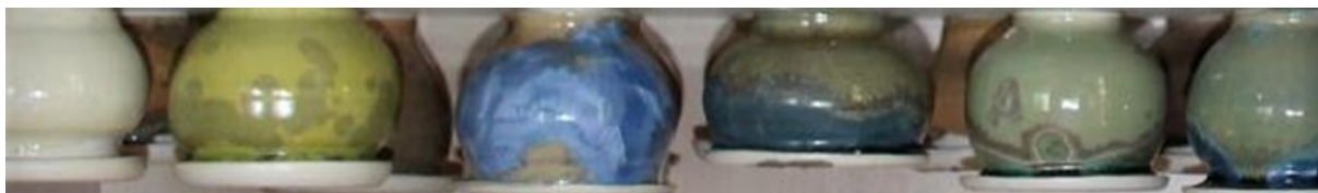
Pots fired upside down to allow glaze runoff to be caught in the rim.
